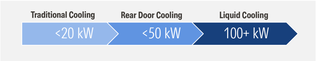
Exhibit 12 Liquid Cooling Is the Most Effective Cooling Solution for AI Data Centers
